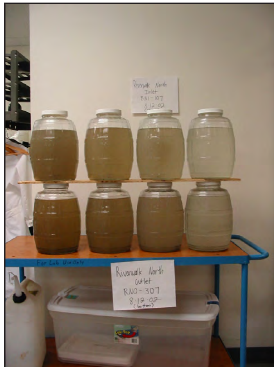
Figure 13. Example of inlet and outlet hydrodynamic-settling device event samples.
